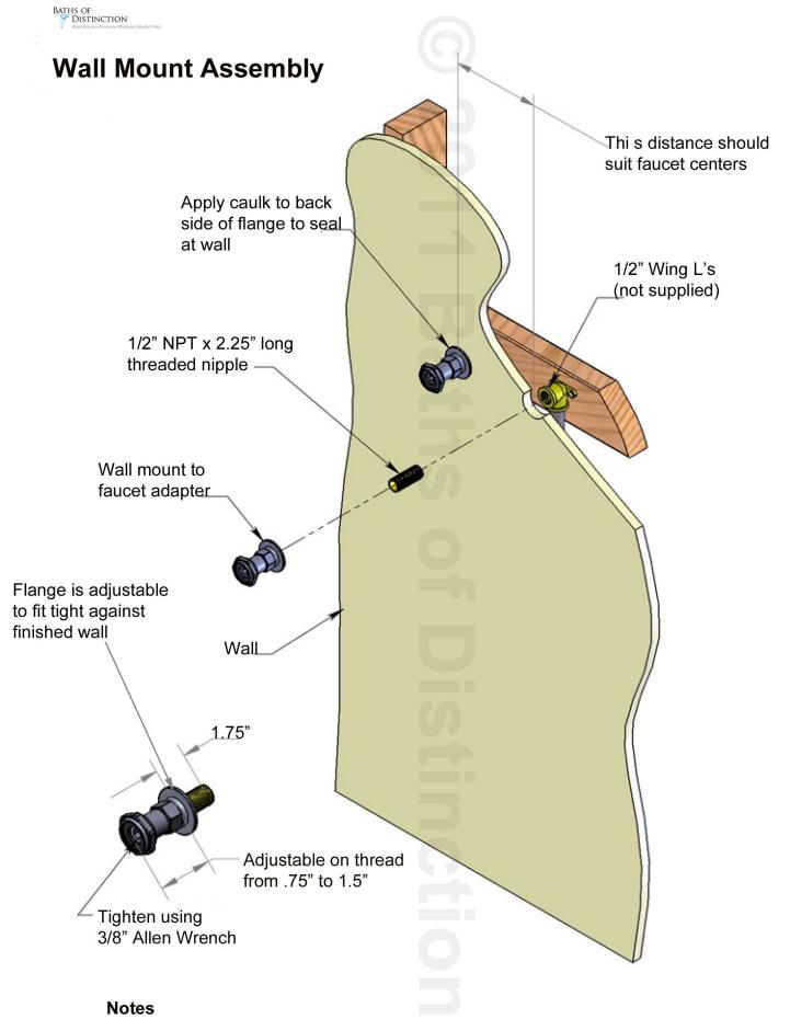
Please take note of the wall mount length and the chosen faucet dimension if installing a tub filler. This will allow you to calculate how far your tub edge can be positioned away from the wall.
